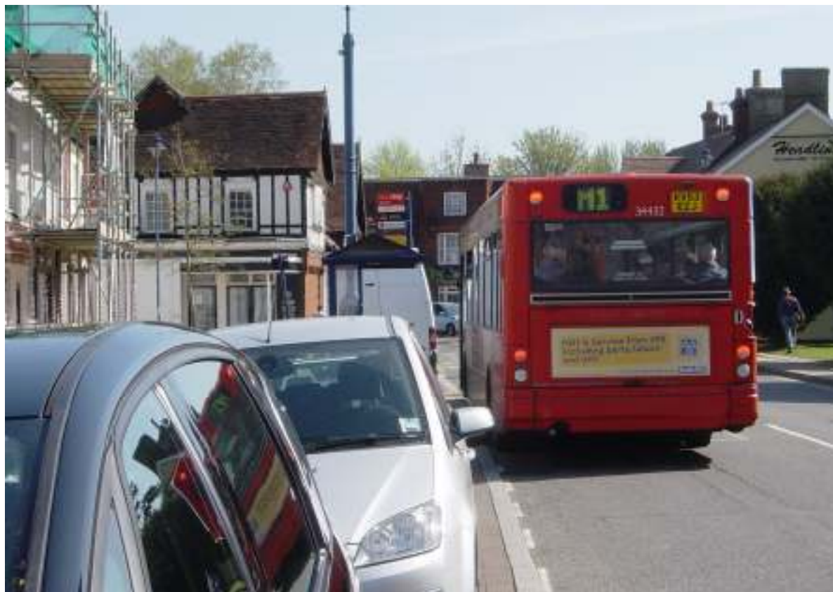
Figure 13, below, shows a particularly perverse example of road layout where adjacent laybys are provided for parked cars in Shefford High Street whilst buses are forced to block the carriageway in front of the traffic lights at a very busy junction. This layout did not happen by accident so the question is asked – what considerations were applied by the highways engineer when the Shefford High Street improvement scheme was implemented!
